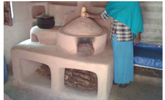
Energy efficient stove made of chikka in the village of Awra Amba (Amhara). It improves the quality of the air inside the house. © Lorenzo Fontana
