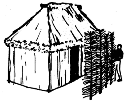
Using woven leaves for improved protection of the walls and for additional closure of the openings. ©Intertext
