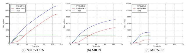
Figure 16: PlanetLab topology: evolution of cumulative data traffic as a function of time
