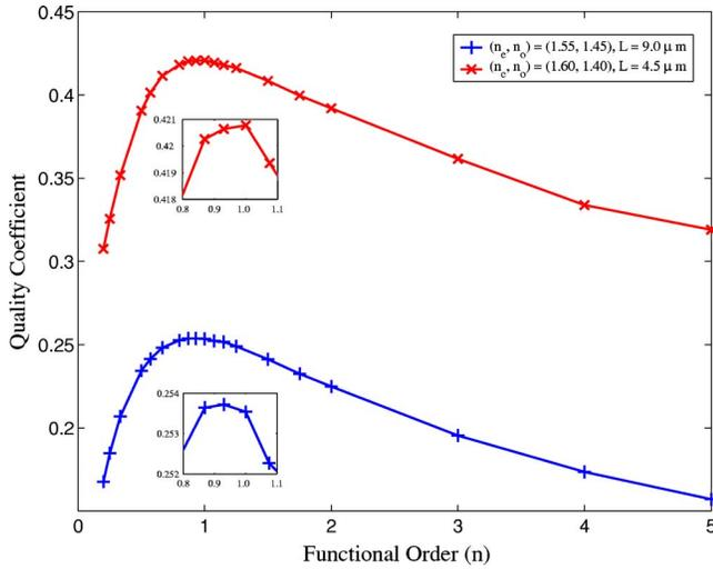
FIG. 9. (Color online) Quality coefficient  $\tilde{R}$  over  $n$  for case A “+”s and case B “x”s. The insets show a magnification of the plots for values of functional order  $n$  around  $n=1$ .
