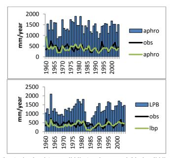
**Fig. 2** Hyetograms (bars), simulated (grey solid line) and measured (black solid line) hydrograms (Nam Khan). Upper figure : Aphrodite database and lower figure Luang Prabang rainfall data.
