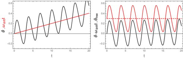
FIG. 3. Comparison of the variation of  $\theta(t)$  with the drift  $\omega_{\text{drift}} t$  [left] and of the residue  $\theta - \omega_{\text{drift}} t$  to the  $\theta(t)$  for the free motion with an arbitrary offset to compare the curves [right]. Parameters:  $\omega_0 = 2$ ,  $a = 0.1$ ,  $V_0 = 0.7$ ,  $x_0 = 1$  m.
