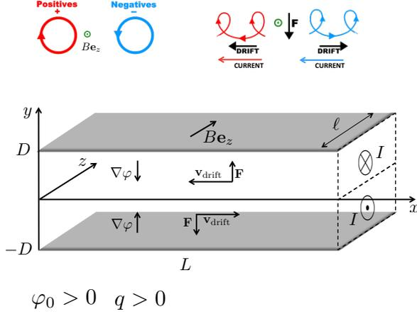
FIG. 7. Experimental design to generate macroscopic current from a fifth force. All quantities are defined in the text and are plotted assuming  $\varphi_0 > 0$  and  $q > 0$ . Top pictures show that particles of opposite charges drift in opposite directions but generate a current in the same direction.
