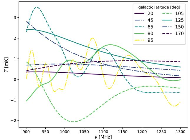
**Figure 2.** Temperature contribution of the polarization leakage as function of frequency, observed along different lines of sight at constant galactic longitude but different latitudes. The leakage has a smooth behaviour at the poles – although dependent on line of sight – and oscillates when closer to the galactic plane.
