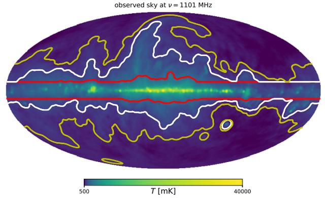
**Figure 12.** Total temperature map of channel  $\nu \in [1100-1102]$  of the simulation. We overplot with solid coloured lines the different masks we use, covering the brightest pixels up to the 10, 25, and 50 per cent of the sky. As expected, it is the galactic plane to be masked out, up to the synchrotron North Polar Spur for larger masks.
