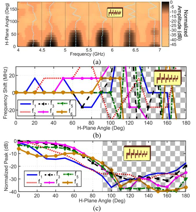
FIGURE 20. (a) Measured frequency-domain response of a high Q-factor depolarizing tag with ground plane [8] as a function of the H-plane angle. In light blue: Detected resonant frequency peaks. (b) Frequency shift of each resonance as a function of the H-plane angle. (c) Normalized amplitude of the signal peaks as a function of the H-plane angle. Tag-reader distance: 20 cm, inside an anechoic chamber.
