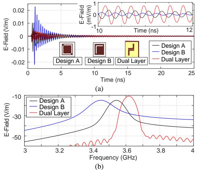
FIGURE 5. (a) Simulated cross-polarization time and (b) frequency domain response of one resonator of the proposed single-layer designs, as well as a dual-layer case.
