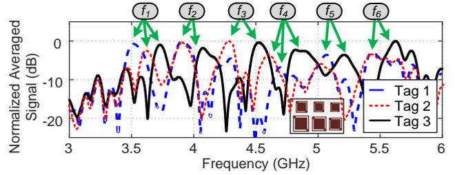
FIGURE 9. Normalized averaged signal of Design A STFT spectrogram, without background and at 25 cm inside an anechoic chamber. Three different tags are shown, where the design dimension  $L$  has been modified to change their resonant frequencies.
