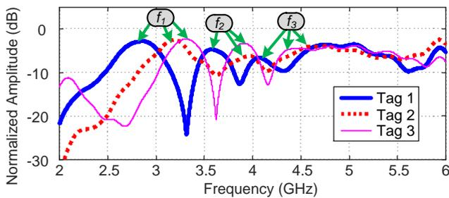
FIGURE 15. Normalized averaged signal of Design B STFT spectrograms in Fig. 14.
