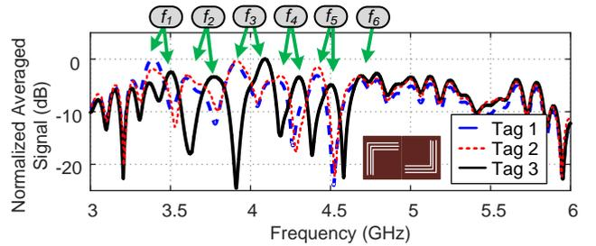
FIGURE 10. Normalized averaged signal of Design B STFT spectrogram, without background subtraction and at 25 cm inside an anechoic chamber. Three different tags are shown, where the design dimension  $L$  has been modified to change their resonant frequencies.
