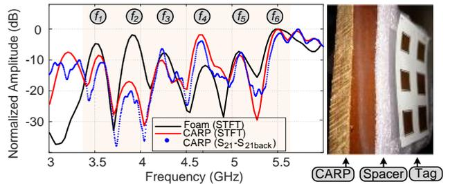
FIGURE 11. Normalized summed signal of Design A STFT spectrogram, without background at 25 cm inside an anechoic chamber. A material (CARP slab with  $\epsilon_r = 5$ ) is attached on the back of the tag. The same measurement without the STFT spectrogram and with background subtraction is given for comparison.
