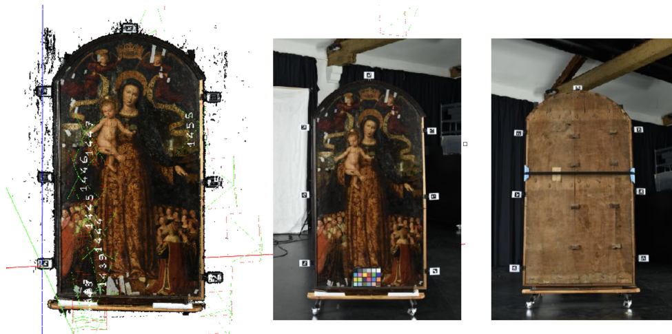
Figure 4. Example of automated scaling and orientation of wood painting base on experimental double sided coded-targets fusion.
