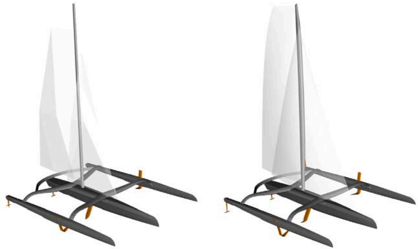
(a) First appendage configuration: small foils and rudders. (b) Second appendage configuration: larger foils and rudders, elevator on centerboard.
