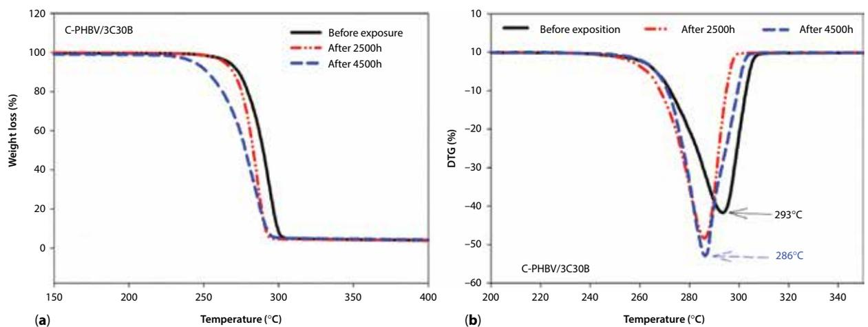
**Figure 4** (a) TGA and (b) DTG curves of C-PHBV/3C30B bionanocomposites before exposure and after 2500 and 4500 hours exposure to accelerated photooxidation.
