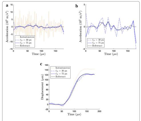
**Fig. 9** Temporal acceleration (**a, b**) and displacement (**c**) measurements of the central node of the mesh. The physical size of one pixel is 500  $\mu$ m. All regularized analyses better capture the accelerations and displacements. For a larger length, the results are very close to the reference solution
