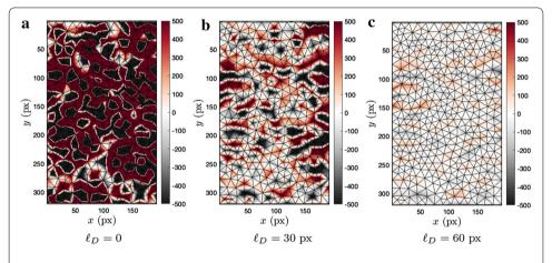
**Fig. 6** Dynamic residuals (in arbitrary units) at  $t=110~\mu s$  with various regularization lengths. The higher the regularization weight (i.e., the higher  $\ell_D$ ), the lower the dynamic residuals
