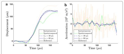
**Fig. 5** Temporal change of displacement (a) and acceleration (b) with three different dynamic regularizations on 180 frames of a 1 Mfps film. The physical size of one pixel is 500  $\mu$ m. The more the DIC analyses are regularized, the closer the measurement to the reference solution
