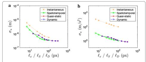
**Fig. 2** Standard displacement (**a**) and acceleration (**b**) uncertainties as functions of the static ( $\ell_S$ ) and dynamic ( $\ell_D$ ) regularization lengths. Comparison with instantaneous and spatiotemporal analyses. The physical size of one pixel is 200  $\mu$ m. The same type of compromise between measurement uncertainty and spatial resolution is found in comparison with instantaneous and spatiotemporal DIC
