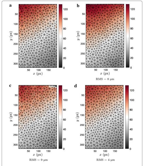
**Fig. 7** Displacement fields (in  $\mu$ m) along x at  $t=85~\mu$ s. **a** Reference solution, **b** instantaneous DIC, **c** spatiotemporal DIC, **d** dynamically regularized DIC ( $\ell_D=75$  pixels). All analyses lead to very low RMS differences between measured displacement fields and the reference solution. The dynamically regularized solution lowers the RMS difference by a factor of 2 in comparison with the other two analyses
