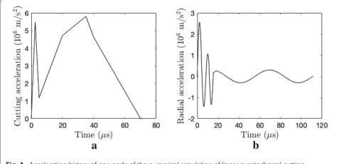
**Fig. 4** Acceleration history of one node of the numerical simulation of linear pyrotechnical cutting. **a** Ignition in the cord of pyrotechnic cutting, **b** shock wave in the plate
