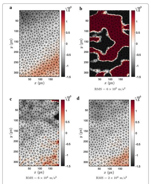
**Fig. 8** Acceleration fields along x at  $t=85~\mu s$ . **a** Reference solution, **b** instantaneous DIC, **c** spatiotemporal DIC, **d** dynamically regularized DIC ( $\ell_D=75$  pixels). The spatiotemporal analysis with no dynamic regularization leads to lower nonphysical fluctuations (RMS difference 10 times lower than instantaneous DIC). Even closer results to the reference solution are obtained with dynamic regularization
