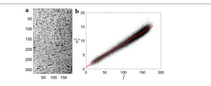
**Fig. 12** a Denoised picture  $\widehat{f}$  in the reference configuration of the virtual test case. **b** Variance of acquisition noise  $\sigma_{\eta}^2$  as a function of the gray level of the denoised picture.  $\widehat{f}$  is constructed by using an actual picture series of the uncertainty analyses. Its definition is  $320 \times 192$  pixels. The acquisition noise is Poissonian since its variance is proportional (solid red line) to the considered gray level
