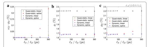
**Fig. 10** Change of  $w_D \varrho_D$ ,  $\varrho_C$  and  $\varrho_R$  (in percentage of the dynamic range) with the regularization length. Two different gray level interpolation schemes were tested. These results prove the efficiency of the dynamic regularization in comparison with the static regularization
