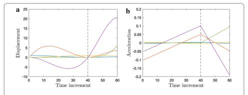
**Fig. 11** Cubic splines (**a**) and 2nd order derivatives (**b**) for 2 elements (temporal node at time increments 0, 40 and 60) when continuities in terms of displacement, velocity and acceleration are prescribed. These results prove that the accelerations are piece-wise linear and continuous in the present implementation
