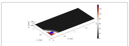
**Fig. 3** Horizontal displacement field (expressed in  $\mu$ m) of the pyrotechnic cutting simulation (when  $t=85~\mu$ s). The blue area shows the ROI analyzed via DIC
