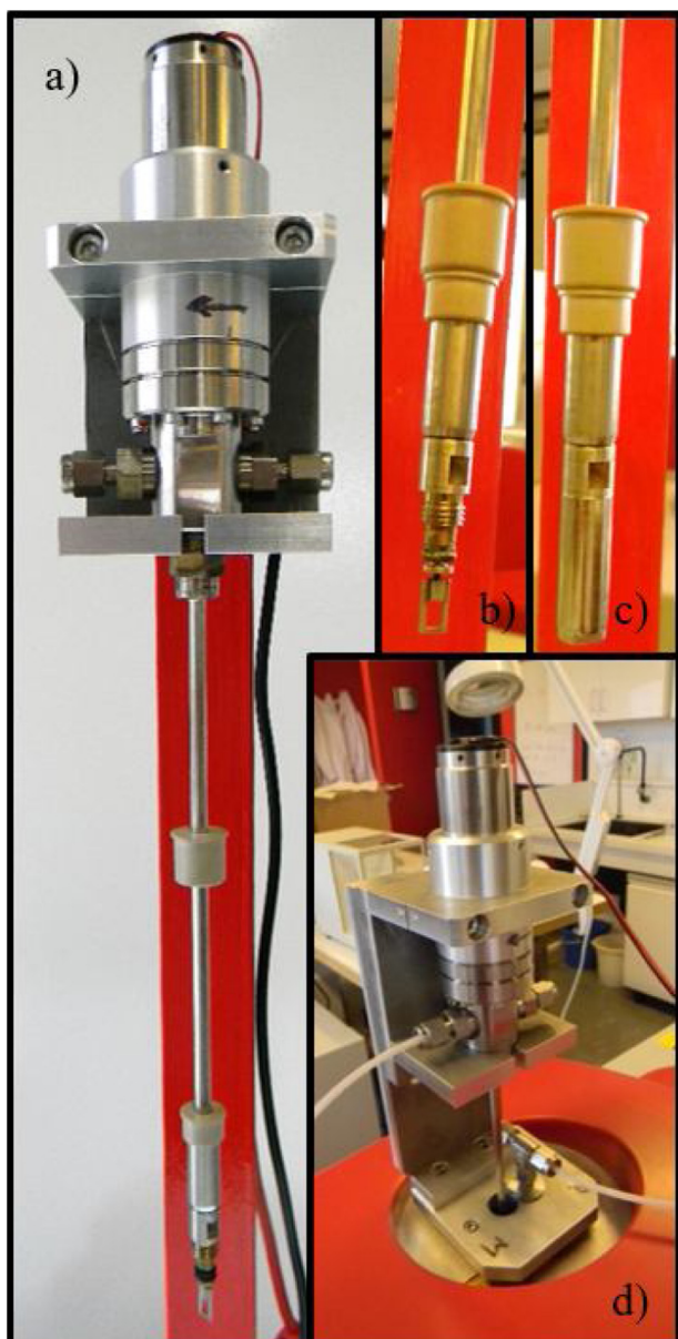
Fig. 2 – Photographs of the prototype: a) full prototype, b) zoom-in on the stirrer and c) the measuring cell before the experiment, d) prototype placed on a Setaram \mu DSC7 evo calorimeter.
