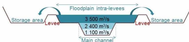
**Figure 1:** Typical cross section of the Garonne River between Tonneins and La Réole, with flow characteristics.
