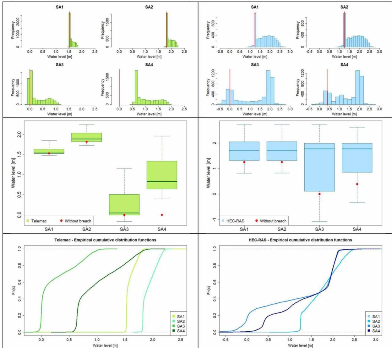
**Figure 6:** Frequency distributions, boxplots and empirical cumulative distributions functions of both meta-models outputs (TELEMAC-2D on the left and HEC-RAS on the right). The red lines/dots represent the simulations without breach.
