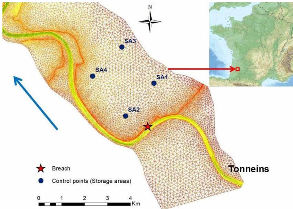
Figure 4: Case study modelling with TELEMAC-2D. Focus on the upper part of the Garonne River.
