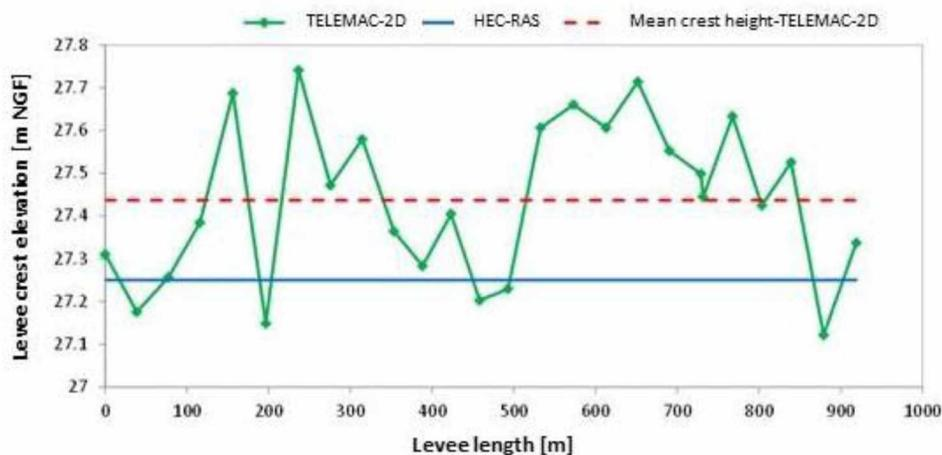
**Figure 5:** Differences between levee modelling in HEC-RAS and TELEMAC-2D.
