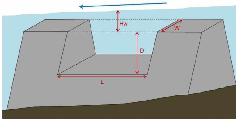
**Figure 3:** Levee breach diagram with length ( $L$ ), depth ( $D$ ), width ( $W$ ) and overflow ( $H_w$ ), as input parameters.
