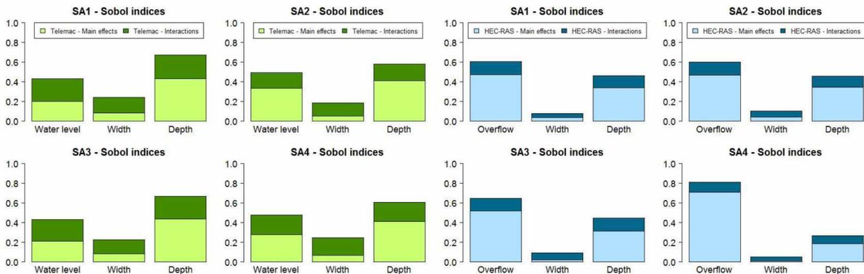
**Figure 7:** Sobol' indices for the four SA and for both models (TELEMAC-2D on the left side and HEC-RAS 1D on the right side). The main effects correspond to the first order Sobol' indices and the whole columns (main effects + interactions) correspond to the total Sobol' indices.
