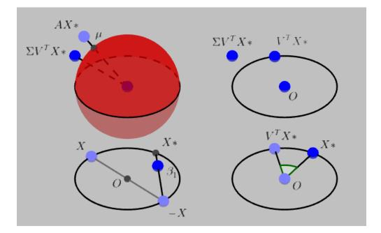
Figure 4: The projection of  $X \in \mathbb{S}^1$  to  $\mu \in \mathbb{S}^2$  counter-clockwise from bottom left. (Bottom Left:) first projection via  $\beta$  when  $\beta$  is inside the circle, (Bottom Right:) Multiplication by  $V^T$ , (Top Right:) Multiplication by  $\Sigma$  and (Top Left:) Final point after multiplication by Uand projecting on the sphere in 3-dimensions.
