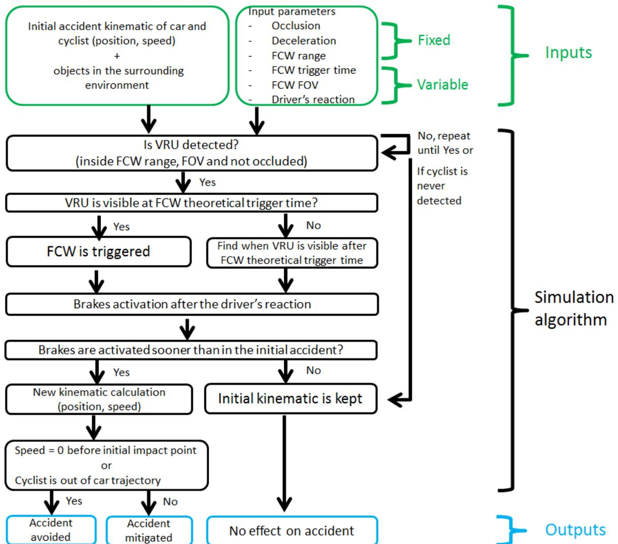
Figure 2: Accident simulation algorithm with FCW effect.
