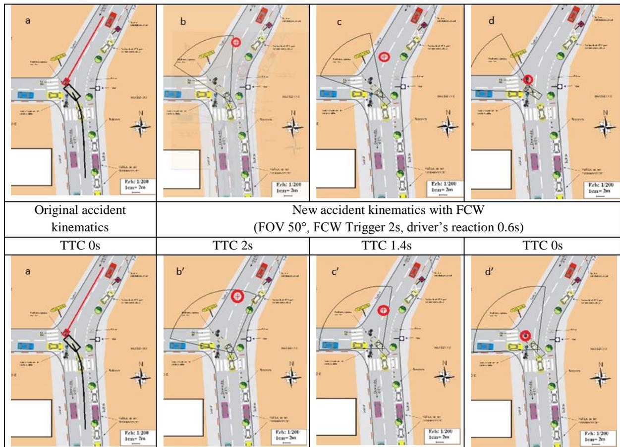
Figure 3: Reconstruction simulation example integrating the effect of FCW. Images a and a' represent the original accident kinematic. Images b, c and d represent a simulation where the FCW has no effect as it is not triggered due to a little FOV (30°). Images b', c' and d' illustrate collision avoidance with a FCW 50° triggered at TTC 2s resulting in a braking activation at TTC 1.4s.
