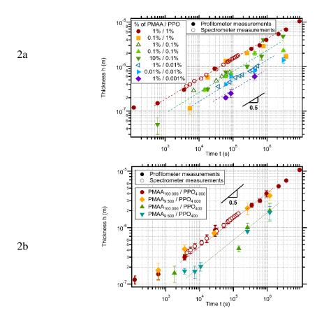
Figure 2. a. Thickness of the PPO-PMAA membrane at the IPM-water interface as a function of time, for varying PMAA and PPO weight percentages between 0.001 wt% and 1 wt%, as measured either with a profilometer (filled symbols) or with a spectrometer (open symbols). The molar masses are:  $M_{\rm w,PPO} = 4000$  g/mol and
