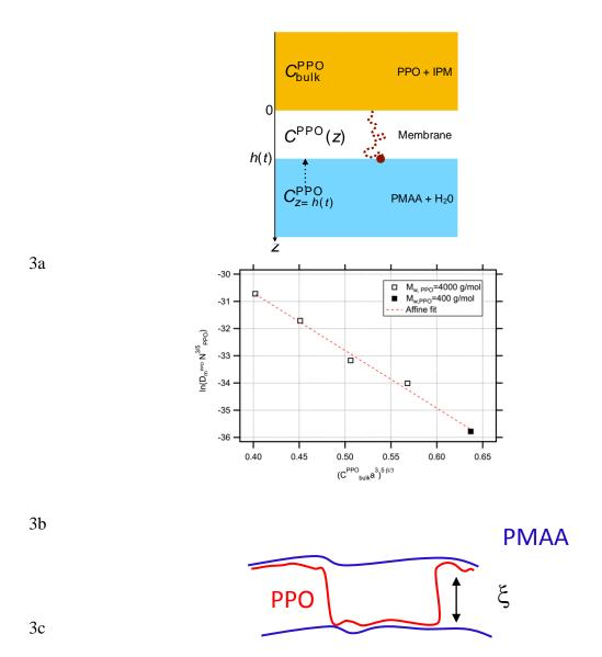
Figure 3. a. Schematic showing the diffusion (red dotted trajectory) of a PPO molecule (red disk) inside a PPO-PMAA membrane (white), from a bulk PPO solution in IPM (z = 0, orange) to the interface with a bulk PMMA solution in water (z = h(t), blue) where PPO-
