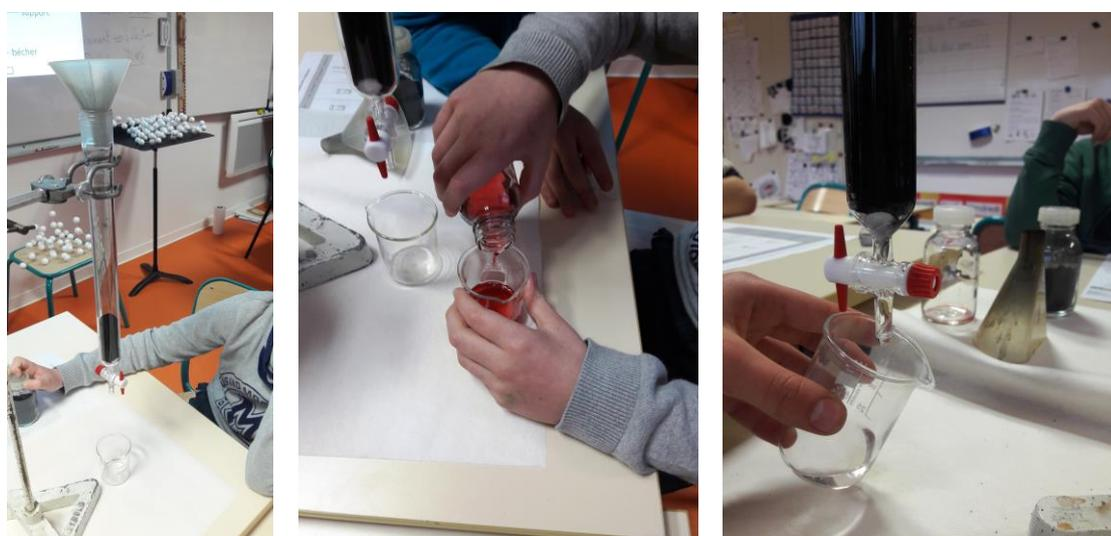
Figure 5. from left to right: preparation of the column, water and grenadine solution, colorless filtrate.
