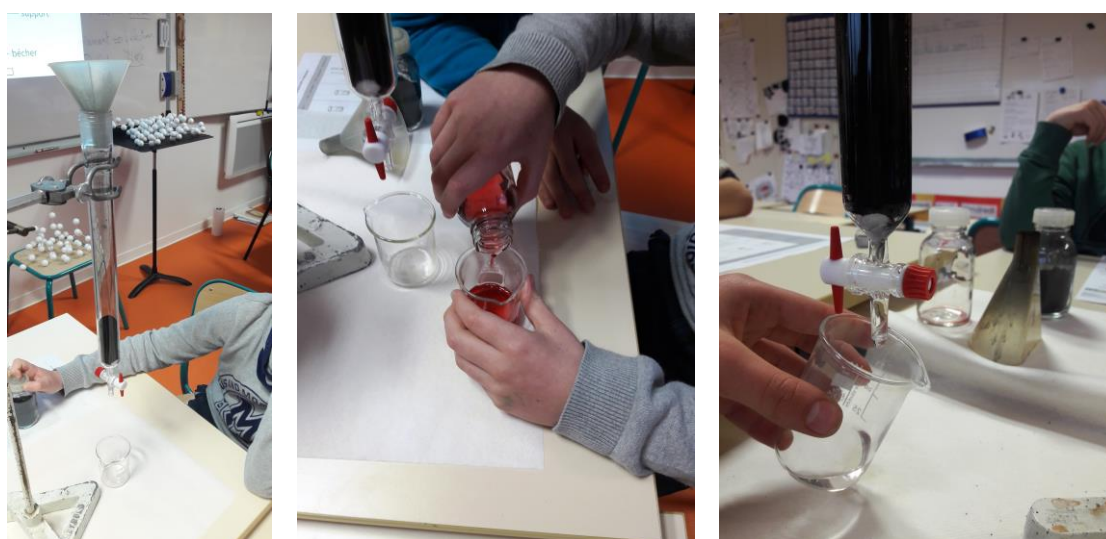
Figure 5. from left to right: preparation of the column, water and grenadine solution, colorless filtrate.
