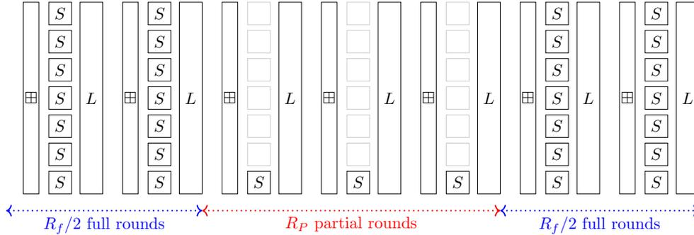
Figure 9: The HADES construction with  $t = 6$ .
