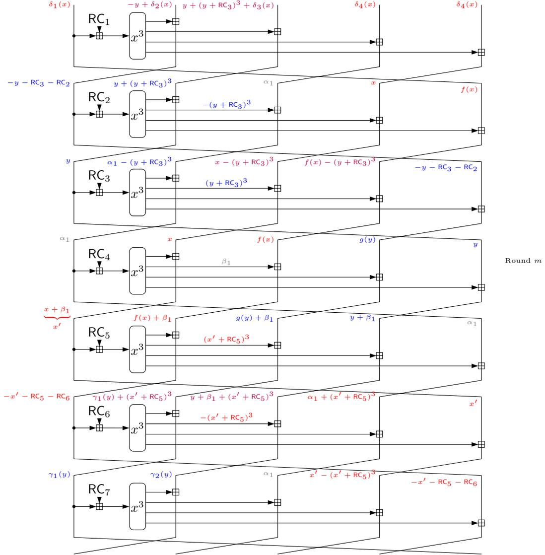
Figure 6: Middle rounds of the zero-sum distinguisher on GMIMC (with  $t = 5$ ) as described in Section 4.2.4.
