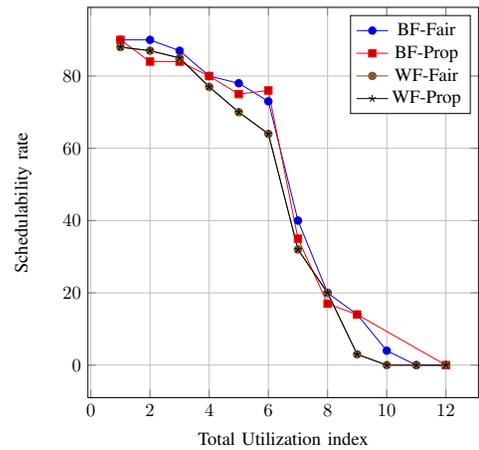
Fig. 4: Heuristics schedulability rate by tasks utilization rate
