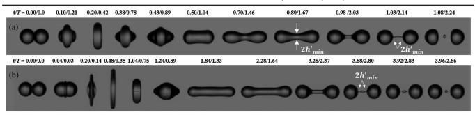
FIG. 1. Collision sequences of (a) two water droplets with D = 2R = 0.3 mm, We = 20.0, and Oh = 0.0089, and (b) silicone oil droplets with D = 0.398 mm, We = 197.3, and Oh = 0.152. The time unit of *t* is a millisecond, and that of *T* is the natural oscillation time  $(\pi/4)\sqrt{\rho D^3/\sigma}$ .
