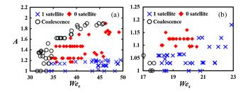
FIG. 6. Formation of satellite droplets in collisions of (a) tetradecane with  $Oh_s = 0.0376$  and (b) water with  $Oh_s = 0.0089$ .  $R_s = 0.3$  mm.
