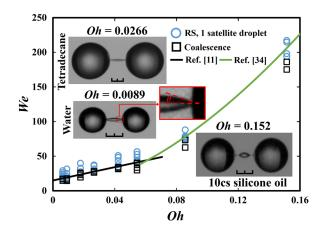
FIG. 2. The boundary between coalescence and RS on the We-Oh diagram. (Insets) Experimental profiles of the drop before breakup. Scaler bar, 200  $\mu$ m.
