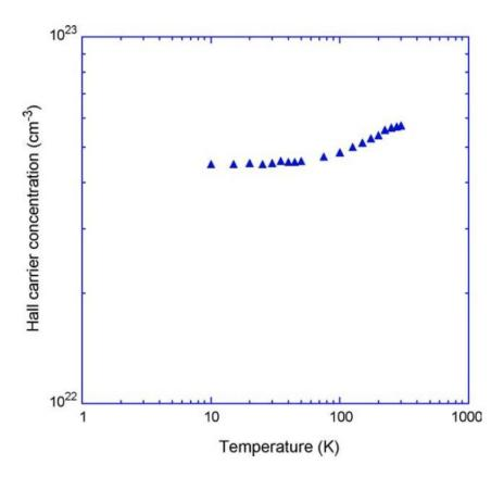
Figure 3: Temperature dependence of the Hall carrier concentration for the film prepared at  $T_s$  = 533 K.
