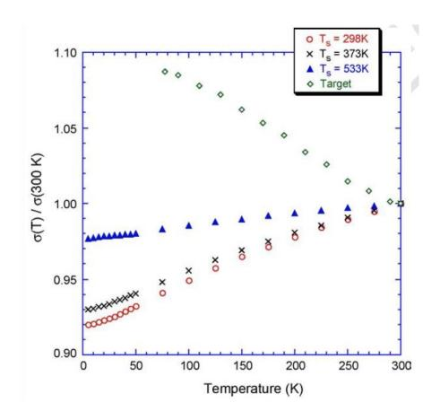
Figure 2: Temperature dependence of the normalized conductivity  $\sigma/\sigma(300~K)$  for the i-  $Ti_{41.5}Ni_{17}Zr_{41.5}$  films and the  $Ti_{45}Zr_{38}Ni_{17}$  target.
