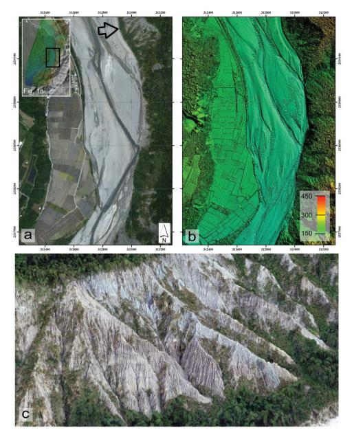
Figure 2. UAV Digital Terrain Model of the Pingting area. (a) Orthorectified photomosaic of the UAV Pingting area. (b) UAV triangular irregular network (TIN) coloured hill-shaded hypsometry. (c) Snapshot of the UAV DTM zoom-in 3D model of the study area where the eroded gully and strata are clearly identifiable from the image. The location of the scene is indicated by the black arrow marker plotted on Figure 2(*a*).
