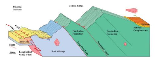
Figure 10. 3D schematic view of the Pingting terraces and the western Coastal Range. The red lines represent the Pingting terraces faults with the line-of-sight displacement rates estimated in this study. The red arrow on the right top corner indicates the direction of convergence between the Philippine Sea Plate and the Eurasian Plate with an estimated rate of about 82 mm per year (Seno et al. 1993).
