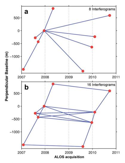
Figure 4. Baseline plot for (a) the persistent scatterer method and (b) the small baseline approach. The red dots represent PALSAR images, while the blue lines indicate the interferograms that are formed. The perpendicular baseline corresponds to the component of the satellite separation distance that is perpendicular to the look direction.
