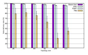
Figure 6: Data packet delivery rates for 10% of nodes as attackers
