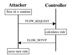
Figure 1: Flase flow request DoS attack
