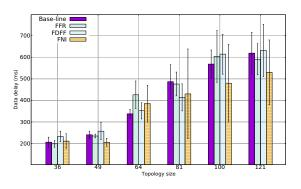
Figure 13: Data packets delay for 10% of nodes as attackers
