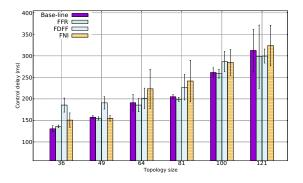
Figure 14: Control packets delay for one attacker
