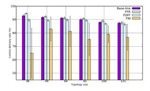
Figure 7: Control packets delivery for one attacker
