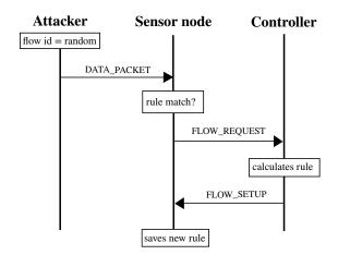
Figure 2: False data flow forwarding DoS attack
