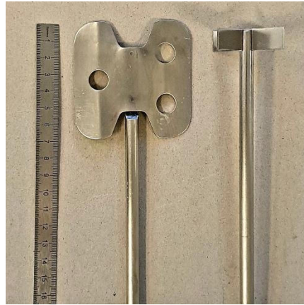
Fig. 1. 3-hole square and 4-bladed impellers.
