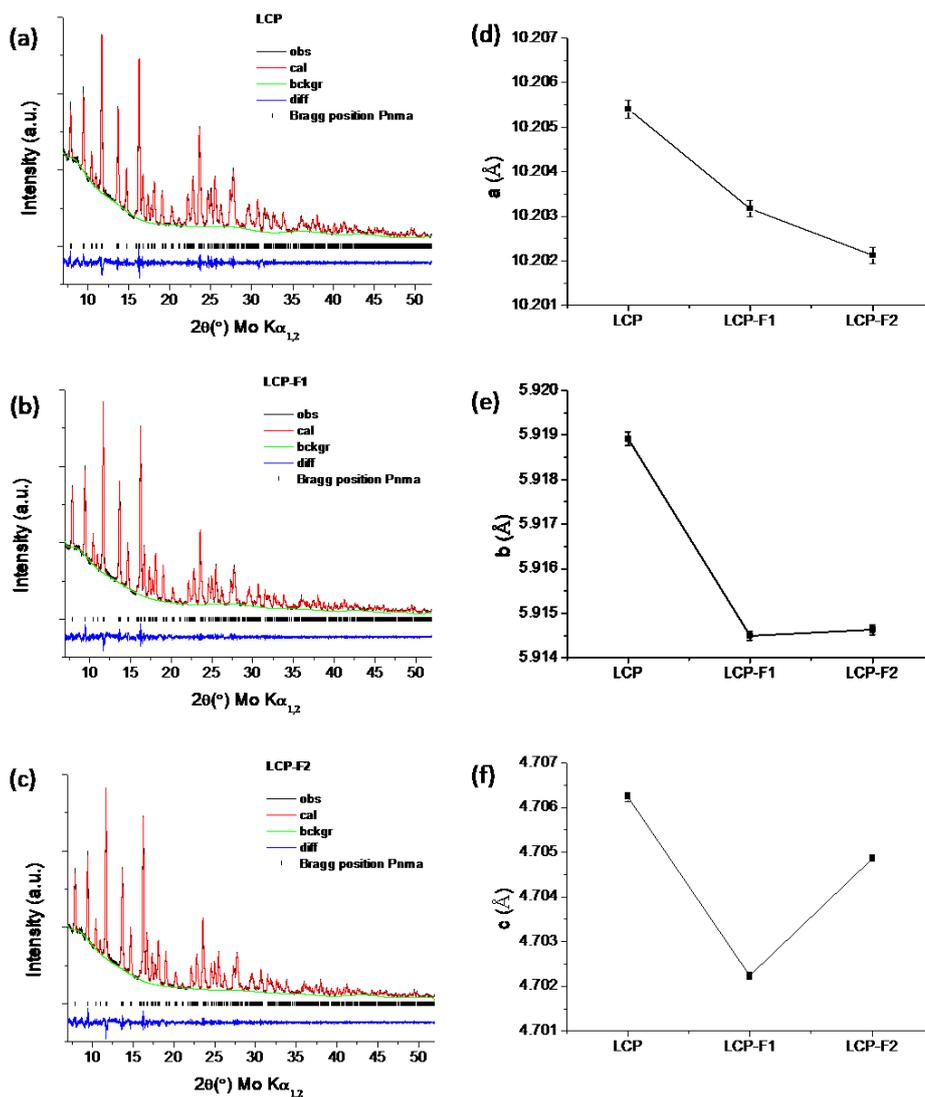
**Figure 1.** Profile fits for powder XRD patterns of (a) LCP, (b) LCP-F1 and (c) LCP-F2 using the Le Bail method. Observed data points are shown in black, with a fitted profile in red and the difference is shown in blue. Tick marks indicate allowed reflections. Refined cell parameters of (d)  $a$ , (e)  $b$  and (f)  $c$ .
