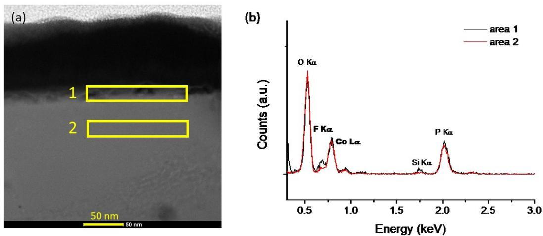
**Figure 3.** a) STEM image of LCP-F2, with surface coated with carbon and platinum (upper side of zone 1, b) EDX spectra of selected zones.
