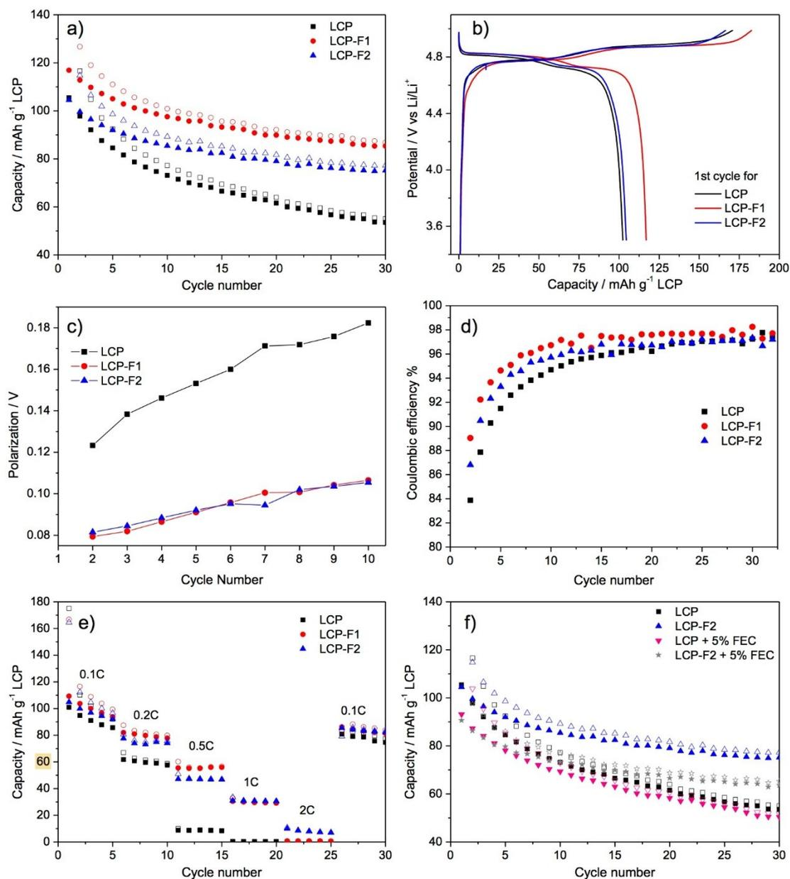
**Figure 5.** Electrochemical performance of the pristine LCP, LCP-F1 and LCP-F2; a) long term cyclability at 0.1 C (16.7 mA g<sup>-1</sup>), b) Galvanostatic profile at 1st cycle at 0.1 C, c) Polarization as a function of cycle number, d) Coulombic efficiency, e) C-Rate performance and f) Comparison with 5% FEC added electrolyte. Open symbols stand for charge capacity and filled symbols for discharge capacity. Long term cyclability result with the error bar can be found in Figure S5.
