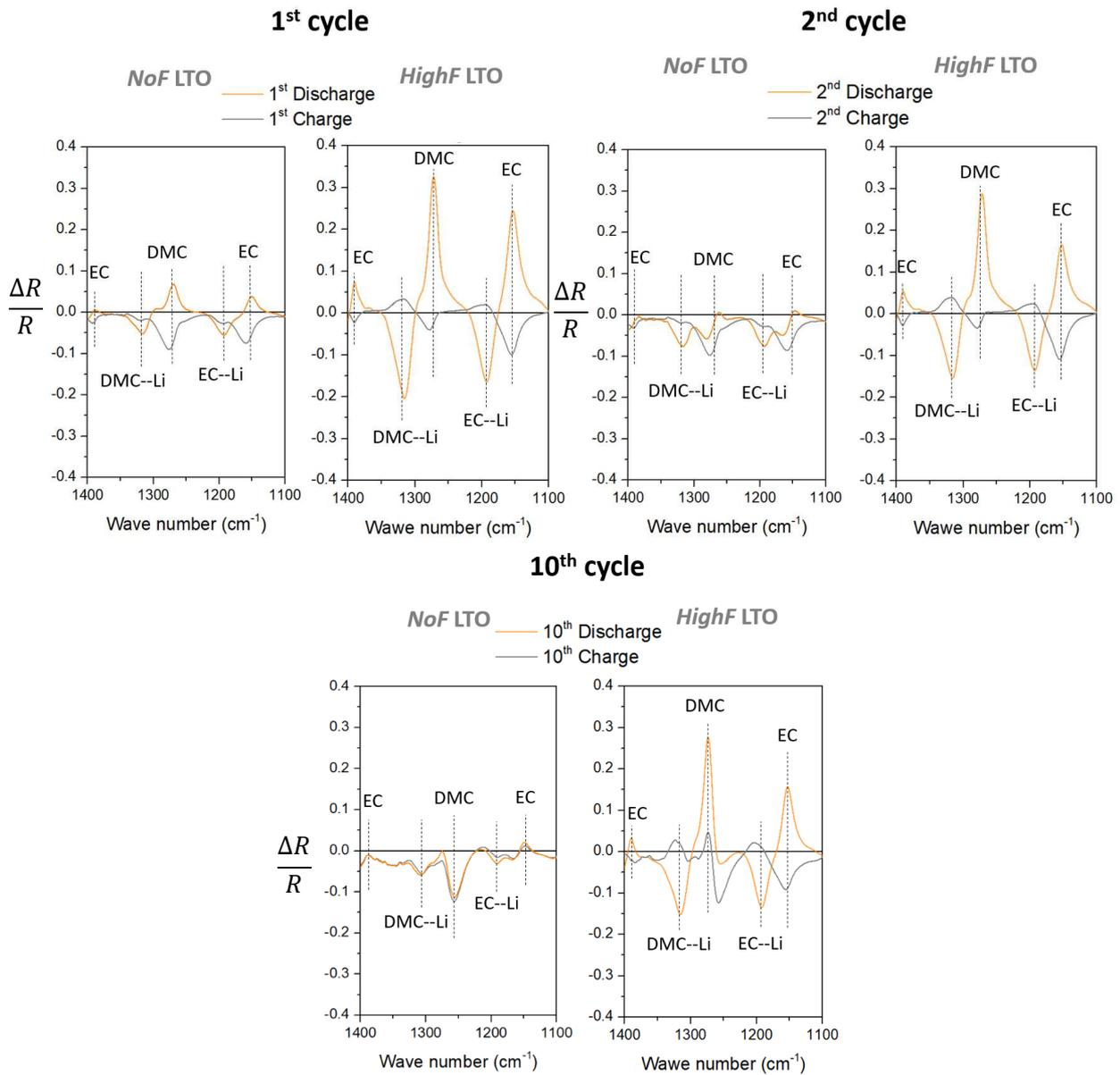
Figure 3 : ATR-FTIR spectra recorded between 1400 and 1100  $\text{cm}^{-1}$  for electrolytes LP30 without additives in the neighborhood of NoF and HighF electrodes for the 1<sup>st</sup>, 2<sup>nd</sup> and 10<sup>th</sup> charge (in grey)/discharge (in orange) cycle. The spectra are displayed in relative intensities: positive bands for formed species and negative bands for consumed species.
