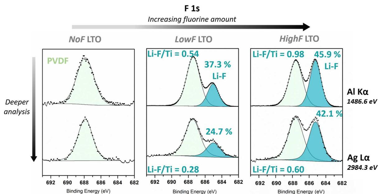
Figure 6 : F1s high resolution spectra recorded for NoF, LowF and HighF fresh electrodes recorded with two X-ray sources Al K $\alpha$  and Ag L $\alpha$ . Relative percentage of Li-F over the fluorine total amount are displayed.
