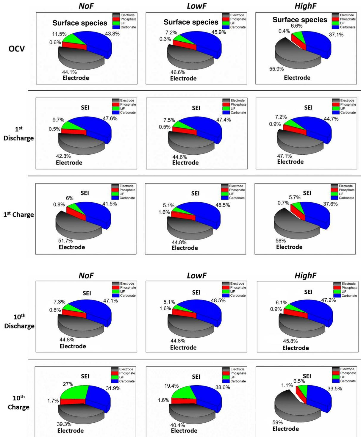
Figure 8 : XPS quantification of Electrodes species (LTO material, carbon black and PVDF) and SEI species (carbonates, LiF and phosphate) after OCV, 1<sup>st</sup> Discharge, 1<sup>st</sup> Charge, 10<sup>th</sup> Discharge and 10<sup>th</sup> Charge.
