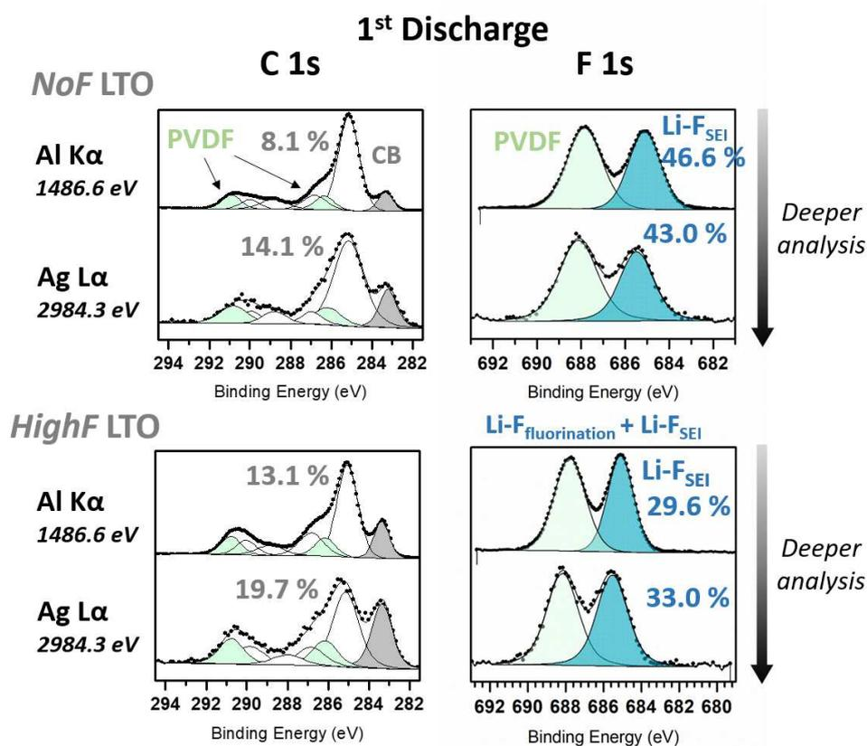
Figure 7 : XPS Al K $\alpha$  and Ag L $\alpha$  C 1s and F 1s spectra recorded after completion of the first discharge for NoF and HighF electrodes. Carbon black (CB) and Li-F environments originated from the SEI formation relative percentages are given.
