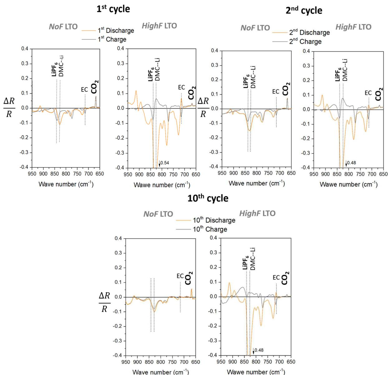
Figure 4 : ATR-FTIR spectra recorded between 950 and 650  $\text{cm}^{-1}$  for electrolytes LP30 without additives in the neighborhood of NoF and HighF electrodes for the 1<sup>st</sup>, 2<sup>nd</sup> and 10<sup>th</sup> charge (in grey)/discharge (in orange) cycle. The spectra are displayed in relative intensities: positives bands for formed species and negatives bands for consumed species.
