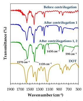
**Figure 3.** FTIR spectra of Ni-MOF-74 samples from before centrifugation (red), after centrifugation 1 (blue), and after centrifugations 1 and 2 (green), with the spectrum of 2,5-dihyroxyterephtalic acid linker (brown) from [30].
