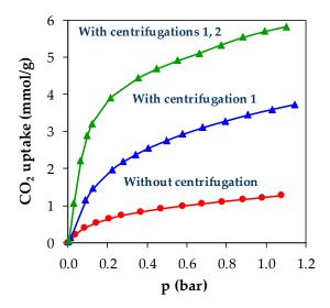
**Figure 2.**  $CO_2$  adsorption isotherms of Ni-MOF-74 samples from the first-batch synthesis after washing repetitions (red) and the second-batch synthesis with centrifugation 1 (blue) and centrifugations 1 and 2 (green), in a pressure range of 0–1.2 bar and at 25 °C.
