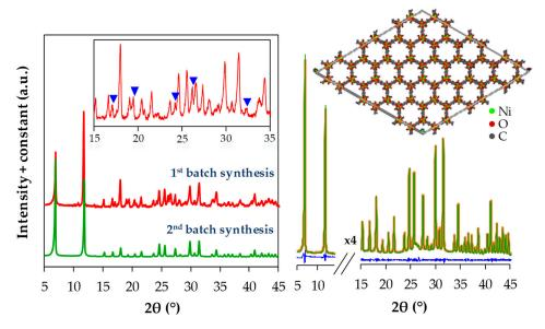
**Figure 4.** (left) Powder X-ray diffraction (PXRD) patterns of Ni-MOF-74 samples from the first-batch synthesis (red) and the second-batch synthesis with centrifugations 1 and 2 (green). (right) Results of Rietveld refinement on the second-batch sample; green, yellow, and blue lines represent experimental data, indexed reflections of molecular structure of Ni-MOF-74, and difference plot, respectively.
