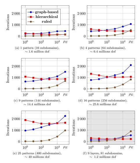
Figure 8: Stratified composite structure (a-e) 8 layers, (f) 9 layers: influence of the heterogeneity ratio  $\rho_E$  on the convergence of the FETI solver for three types of decomposition and an increasing number of subdomains.
