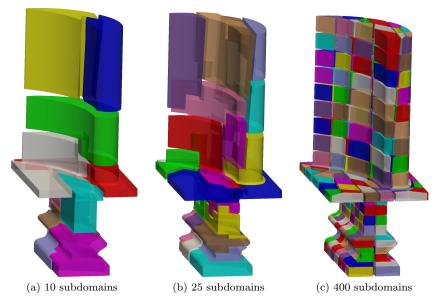
Figure 10: Hierarchical decompositions of the turbine blade
