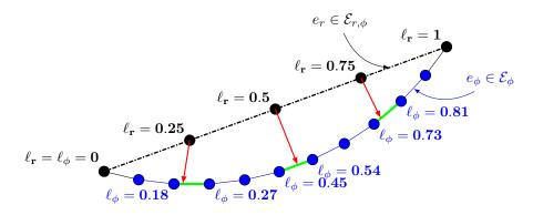
Figure 6: Projection of the edge of  $e_r \in \mathcal{E}_{r,\phi}$  (in dashed black line) on the corresponding edge  $e_{\phi} \in \mathcal{E}_{\phi}$  (in solid blue line),  $\ell_r$  and  $\ell_{\phi}$  are the normalized curvilinear abscissa. The green lines are the segments where the condition  $\ell_{r,k} \in [\ell_{\phi,K}, \ell_{\phi,K+1}]$  is satisfied.
