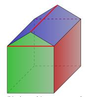
(b) A resulting coarse mesh  $(\mathcal{T}_c, \mathcal{F}_c, \mathcal{E}_c)$ . Red edges corresponds to non-physical edges lying in  $\mathcal{E}_{c,\mathcal{F}}$ , other edges are in  $\mathcal{E}_{c,\phi}$ . Here, the only non-physical coarse face is the one shared by the hexahedron and the prism.
