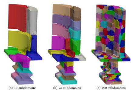
Figure 11: Graph-based decompositions of the turbine blade
