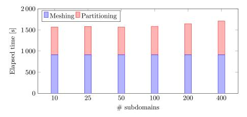
Figure 13: Elapsed time of the sequential meshing and partitioning of the blade with approximately  $1.6{\rm M}$  of nodes
