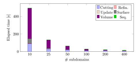
Figure 12: Elapsed time of the meshing process versus the number of subdomains for a constant size of the global problem
