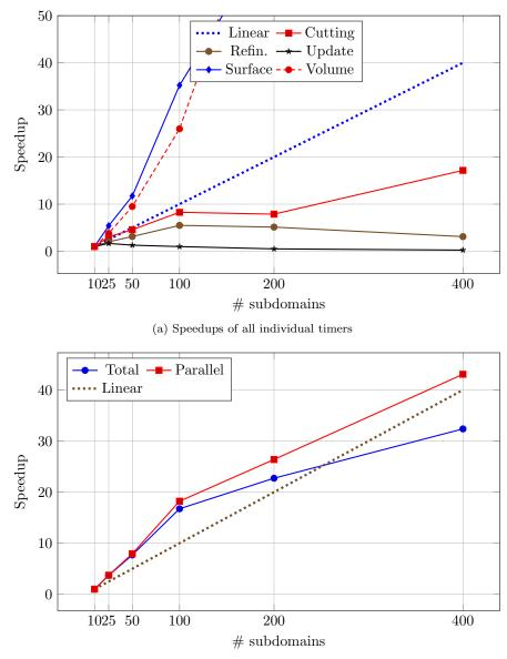
(b) Speedup of cumulated timers (Parallel={Cutting, Refin., Update, Surface, Volume}, Total={Parallel, Seq.})
