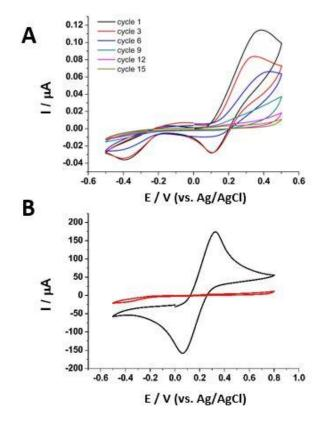
Figure 2: Typical CV profiles for the electropolymerization of a non-imprinted pDA film in phosphate buffer pH 7.4 using up to 15 cycles. A colour code is used to distinguish the CV profiles as function of the number of cycles. (B) Signal blockage of 5 mM ferro/ferricyanide solution upon electropolymerized pDA film on a gold electrode (red) compared with a cyclic voltammogram on a bare electrode (black).
