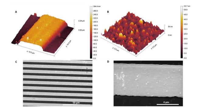
Figure 5: AFM profiles (A, B) and SEM images (C, D) of IDEAU5 coated with p(DA) using 15 cycles. (A) and (C) correspond to the bare electrode whereas (B) and (D) correspond to the imprinted polymer film.
