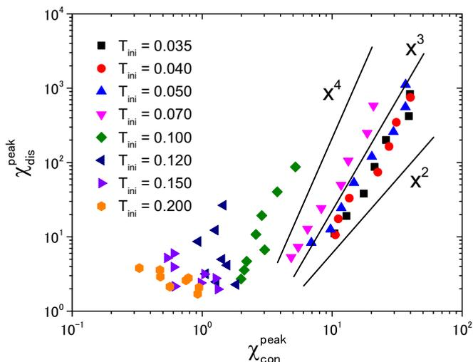
FIG. 5. Parametric (log-log) plot of the peak values of the disconnected and connected susceptibilities for all system sizes and preparation temperatures. For  $T_{\text{ini}} \lesssim 0.10$  the logarithm of the disconnected susceptibility grows with the logarithm of the connected one.
