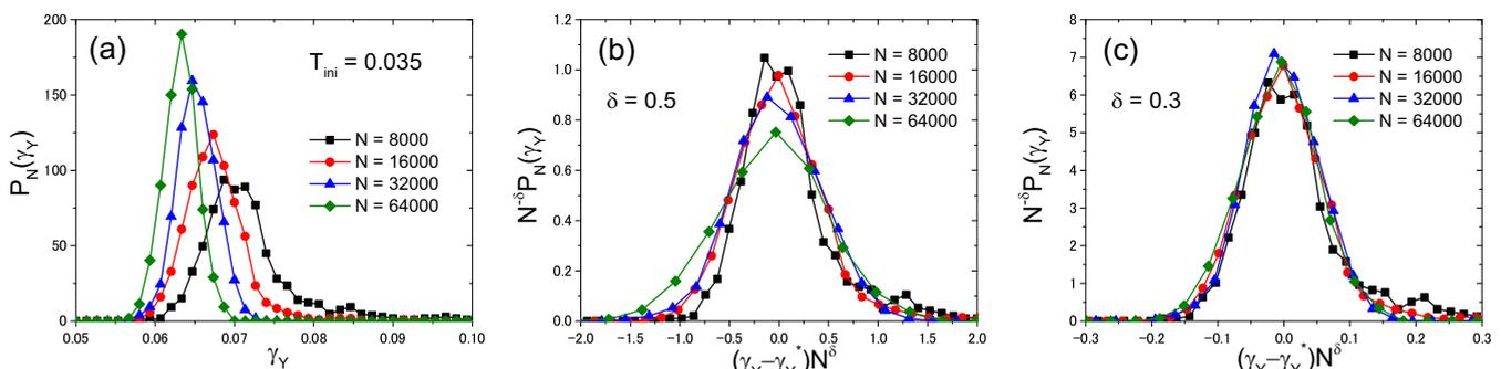
FIG. 6. (a) Probability distribution of  $\gamma_Y$  determined by the position of the largest stress drop,  $\Delta\sigma_{\text{max}}$ . (b), (c) Scaling analysis assuming Eq. (A1) with  $\delta = 0.5$  (b) and  $\delta = 0.3$  (c).
