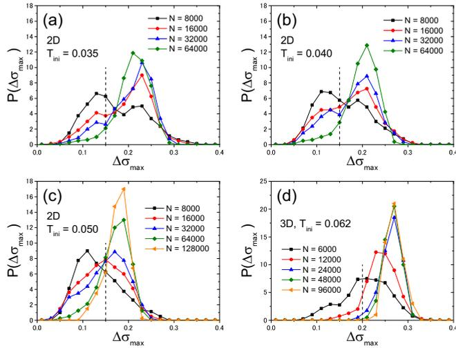
FIG. 7. Probability distribution of the maximum stress drop  $\Delta\sigma_{\max}$  at  $T_{\text{ini}} = 0.035$  (a),  $0.040$  (b), and  $0.050$  (c) in 2D. The 3D model at  $T_{\text{ini}} = 0.062$  is shown in (d) for comparison. The vertical dashed lines indicates the chosen cutoff separating typical and anomalous samples.
