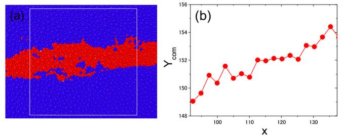
FIG. 10. (a) Snapshot representing the particles belonging to a shear band (shown in red) for a 2D sample at a strain  $\gamma = 0.07$ . The rest of the sample is essentially an elastic body and is shown in blue. (b) The  $y$  coordinate of the center of mass of the shear band for each bin along the  $x$  direction.
