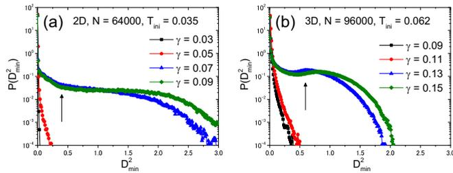
FIG. 9. Probability distribution of the particle nonaffine (squared) displacement  $D_{\min}^2$  in 2D (a) and in 3D (b) for several values of the strain  $\gamma$  covering the regimes before and after yielding. The vertical arrows indicate the threshold above which particles are considered as belonging to a shear band. We have chosen  $D_{\min}^2 > 0.4$  in 2D and  $D_{\min}^2 > 0.59$  in 3D.
