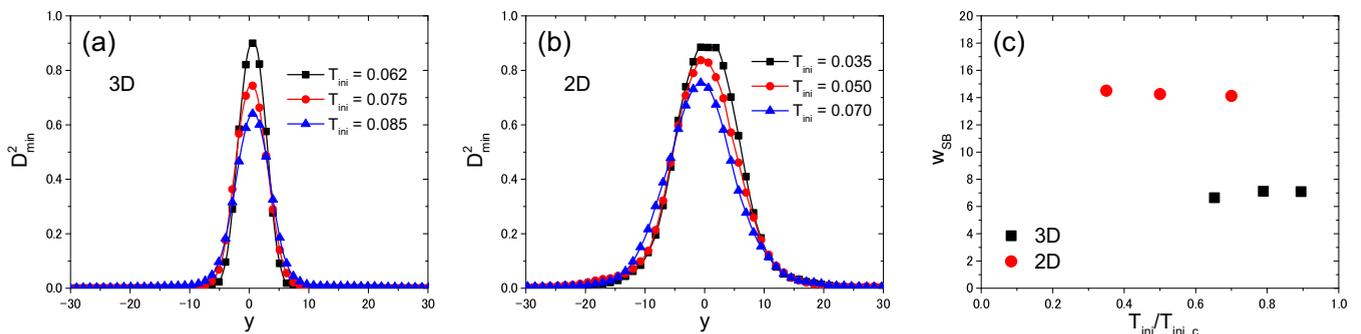
FIG. 8. Averaged  $D_{\text{min}}^2$  profile along the direction perpendicular to the shear band for several preparation temperatures in 3D (a) and 2D (b). (c) Width of the shear band as a function of the normalized preparation temperature  $T_{\text{ini}}/T_{\text{ini},c}$ .
