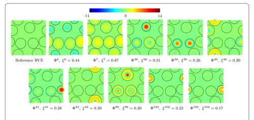
**Fig. 3** Eigenvectors  $\underline{\Phi}_{\mu}$  and  $\underline{\Phi}_{u}$  are shown in a coupled manner: the color map indicates the chemical potential value and the corresponding mechanical modes are indicated by the geometry change (swelling or shrinkage) of the inclusions. The displacement field is scaled 5 times relative to the reference configuration. The quantitative contribution  $\xi^{k}$  of the mode is defined in Eq. (116)
