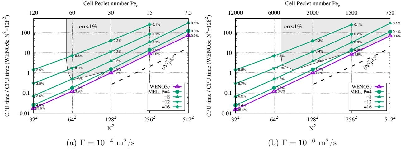
Figure 12: Normalized computational cost for the different schemes as a function of the total unknowns  $N^2$ . The gray area represents solutions with less than 1% relative difference (numerical values) with the reference solution.
