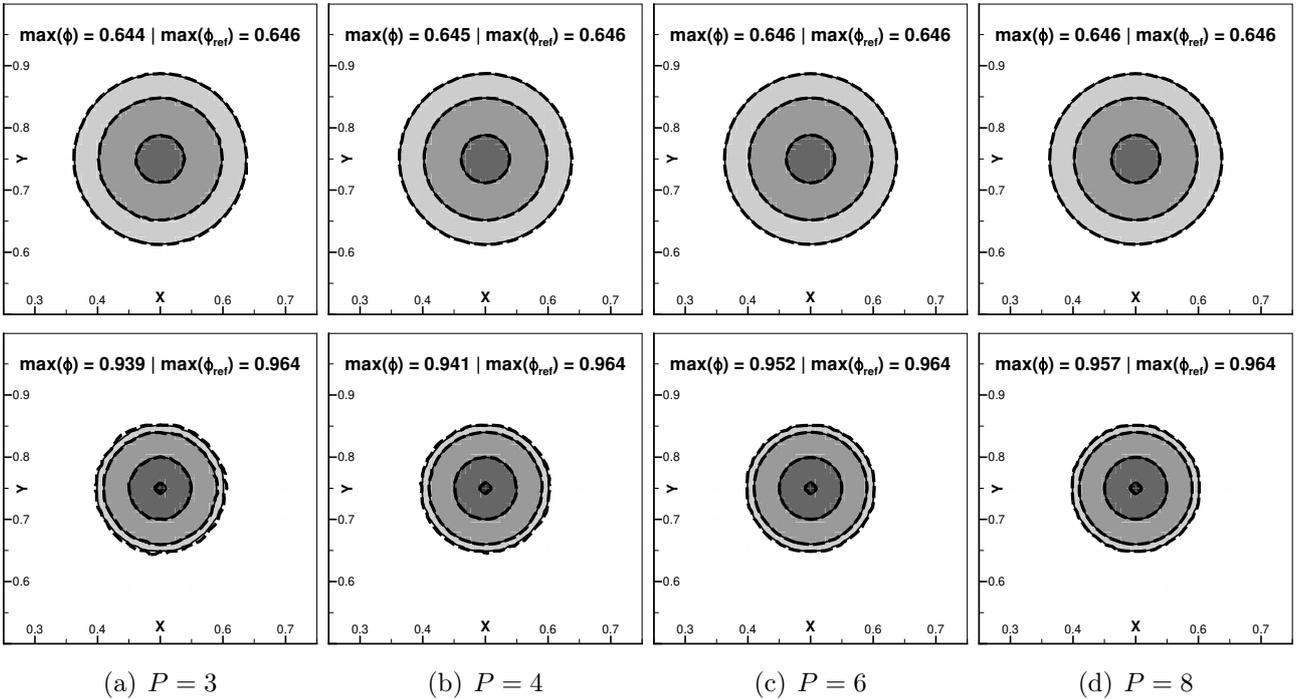
Figure 7: Zoom on the numerical (black dashed lines) and reference solutions (filled) after one turn for different values of  $P$  on a  $N^2 = 128^2$  mesh and for  $\Gamma = 10^{-4}$  (top row) and  $\Gamma = 10^{-6}$  m<sup>2</sup>/s (bottom row). The CFL is set to 0.5. Same iso-lines as in Fig. 6 are shown.
