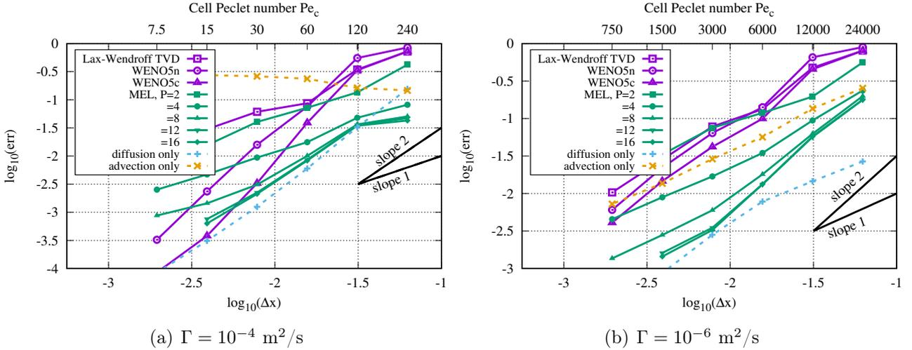
Figure 10: Evolution of error with the space step with  $\Delta x = 1/N$ ,  $N = 16$  (most right points), 32, . . . , 512 for different diffusivity values. The CFL condition is kept at 0.5. For guidance, the top horizontal axis gives the cell Péclet number  $Pe_c$ .
