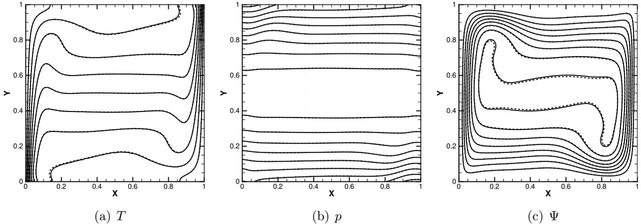
Figure 15: Iso-lines of the temperature  $T$ ,  $\delta T = 0.1$ , pressure variation  $p$ ,  $\delta p = 10^5$ , and stream function  $\Psi$ ,  $\delta \Psi = 2 \times 10^{-3}$ , fields obtained with the MEL scheme (plain lines) and centered (dashed lines) schemes. The  $128^2$  mesh is refined near walls with a Gauss-Lobatto distribution of the cell centers.
