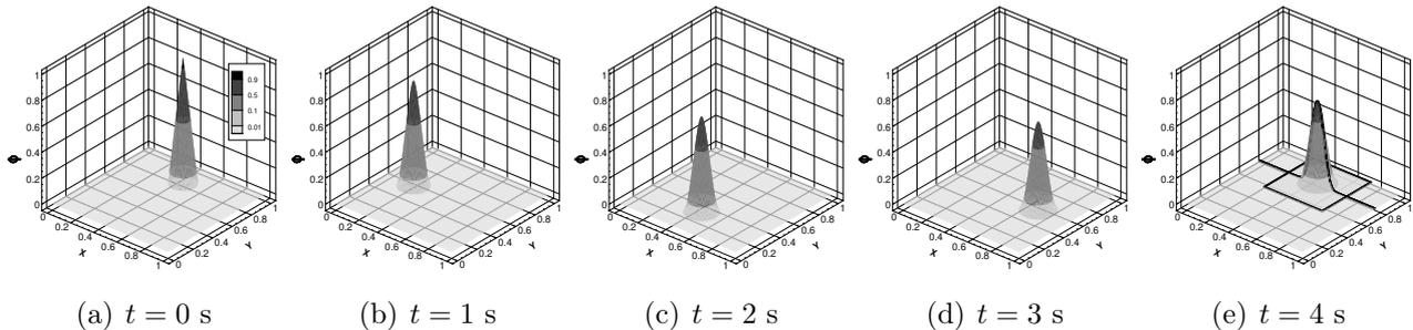
Figure 5: Reference solution for times  $t = 0, 1, 2, 3$  and  $4$  s and for  $\Gamma = 10^{-4}$ . Iso-values are  $0.9, 0.5, 0.1$  and  $0.01$ . Square and dot-dashed line presented in Fig. 5(e) show the zones in which the solution presented in the next section.
