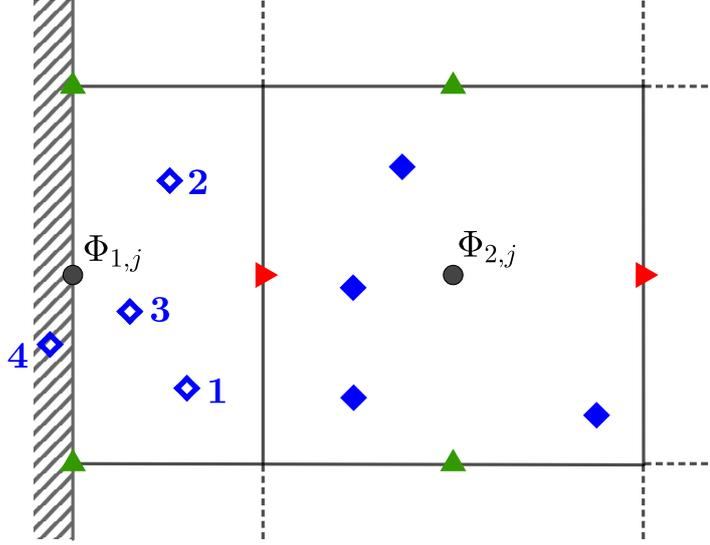
Figure 3: Zoom near a physical boundary. The update (Eq. (11)) of particle local information  $\phi$  in boundary cells (blue empty diamonds) is modified. Markers outside the domain boundaries are turned off during the time integration process.
