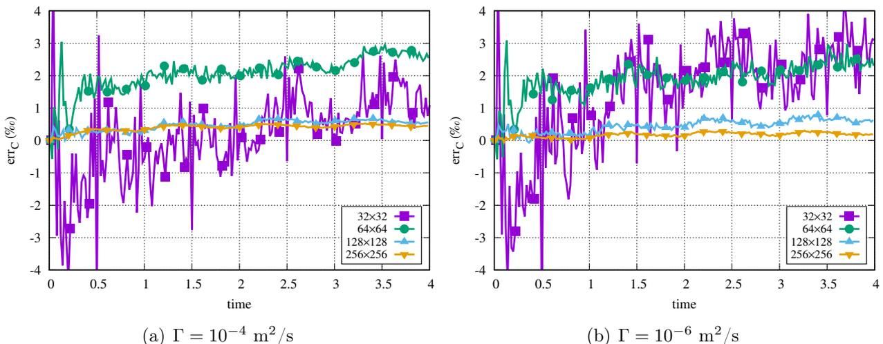
Figure 8: Evolution of the global conservation estimator  $err_C$  over time for different meshes. The averages are done over  $N_R = 128$  runs. (A study on the mean value and variance has been performed on the  $64^2$  mesh and over 2048 runs and has shown a convergence around the  $N_R = 128$  value.)
