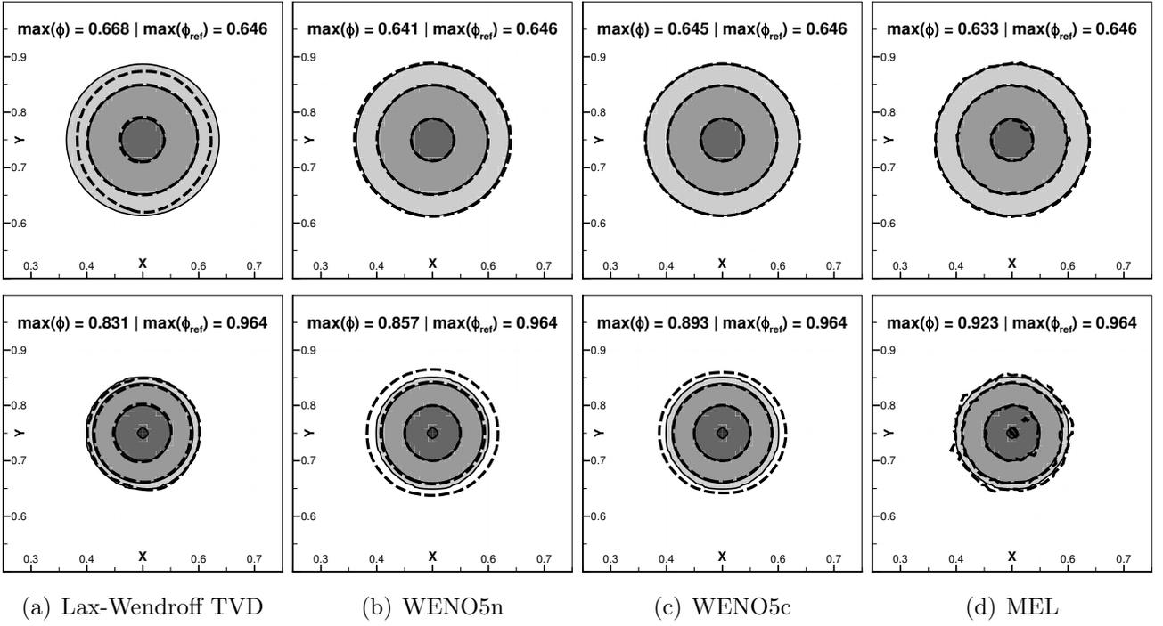
Figure 6: Zoom on the numerical (black dashed lines) and reference solutions (filled) after one turn for different schemes on a  $N^2 = 128^2$  mesh and for  $\Gamma = 10^{-4}$  (top row) and  $\Gamma = 10^{-6}$  m<sup>2</sup>/s (bottom row). The CFL is set to 0.5. Iso-lines are, starting from the peak center, equal to 0.9, 0.5, 0.1 and 0.01 (iso-line 0.9 is not present for  $\Gamma = 10^{-4}$  m<sup>2</sup>/s).
