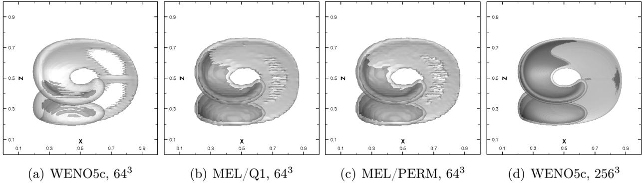
Figure 14:  $XZ$  view of iso-surfaces  $\Phi = 0.2$  (gray) and  $0.9$  (dark gray) for schemes (a) WENO5c on a  $64^3$  mesh, MEL with the particle density number  $P = 4$  on  $64^3$  meshes for Q1 (b) and PERM (c) spatial interpolations and (d) WENO5c on a  $256^3$  mesh, which is used as a reference. The time is  $t = 1$  second, the diffusivity is  $\Gamma = 10^{-6}$  m<sup>2</sup>/s and the CFL = 0.5.
