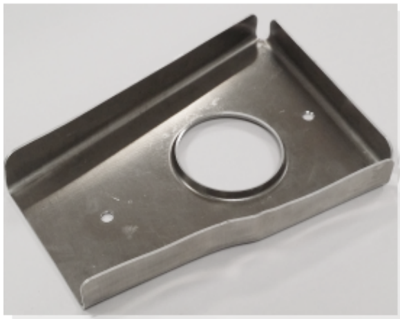
(a) Isometric view of a AA2024-T4 formed part
