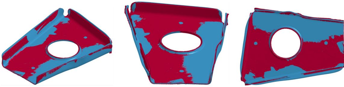
Figure 31: Superposition of the digitized experimental deformed shape (in red) and the computed deformed shape (in blue).
