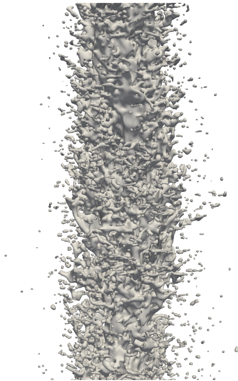
FIG. 12: Zoomed view of the original Spray A configuration case presented in Figure 11. Surface representation based on the Level Set function 0 isocontour.
