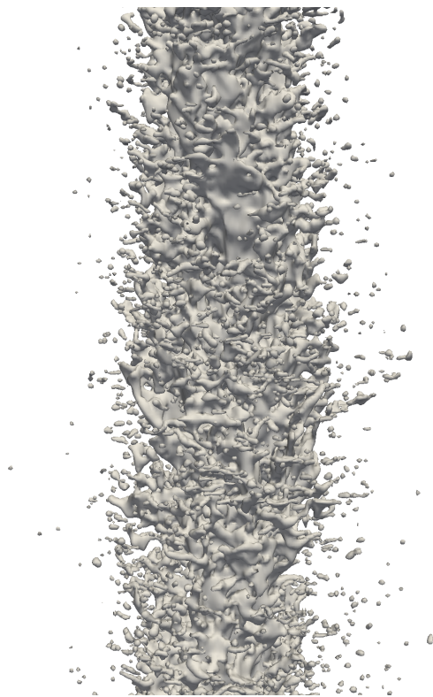
FIG. 12: Zoomed view of the original Spray A configuration case presented in Figure 11. Surface representation based on the Level Set function 0 isocontour.
