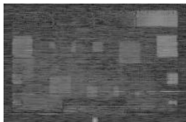
Figure 3 (a) 100 GHz radar scan of a glass fiber composite test sample displaying inclusions (b) 300 GHz radar scan of the same test sample.
