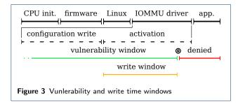
after IOMMU activation in the IOMMU driver activation phase. Right after IOMMU activation, DMA is denied for malicious peripherals. The write window depicts the short interval of time during which the IOMMU configuration is fully placed in DRAM and is vulnerable.
