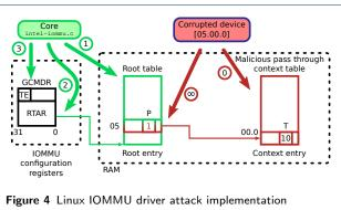
When Linux begins its execution, it first writes its own root table (steps 1 and 2). The second step to be performed by the attacker is to overwrite the root table entry associated to her device. If the corrupted device is connected to logical bus 5, the sixth entry has to be overwritten before the IOMMU activation through bit TE.
