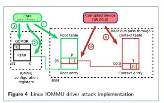
When Linux begins its execution, it first writes its own root table (steps 1 and 2). The second step to be performed by the attacker is to overwrite the root table entry associated to her device. If the corrupted device is connected to logical bus 5, the sixth entry has to be overwritten before the IOMMU activation through bit TE.
