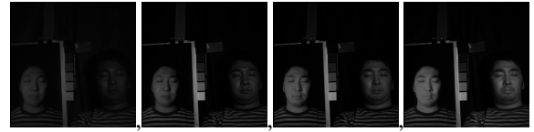
Fig. 7. face photo and genuine face at 400nm, 500nm, 600nm, 700nm
