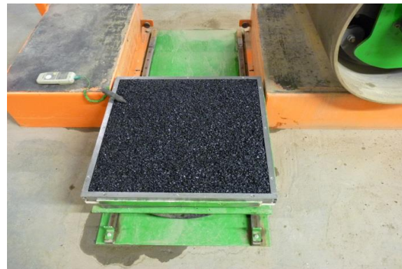
Figure 5. Moulds used to prepare slabs
