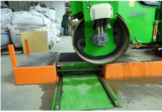
Figure 6. Drum roller compacting a specimen
