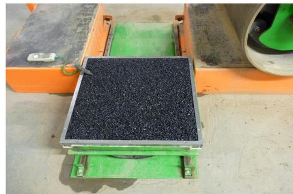
Figure 5. Moulds used to prepare slabs
