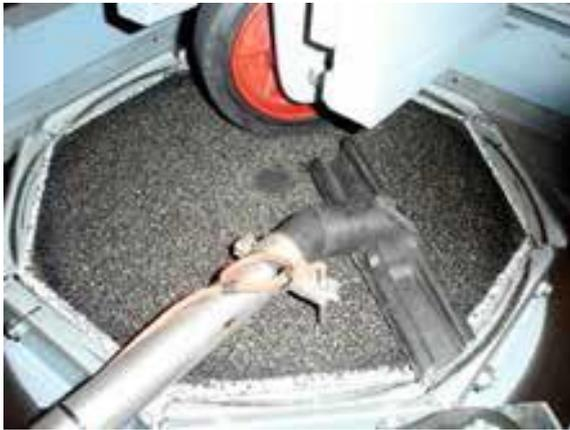
Figure 3. Rotating Surface Abrasion Test (RSAT)
