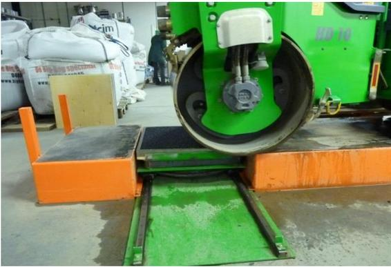
Figure 6. Drum roller compacting a specimen
