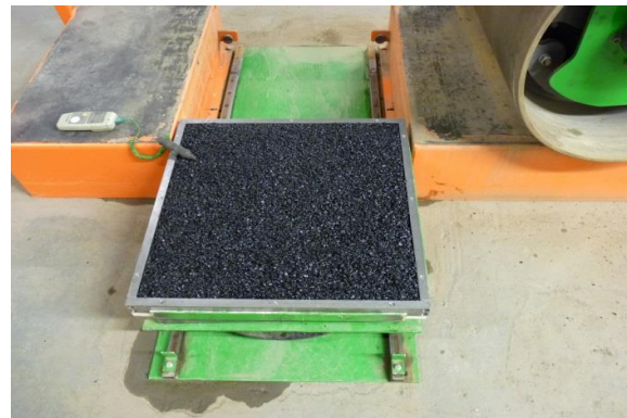
Figure 5. Moulds used to prepare slabs
