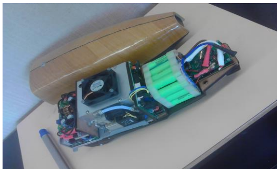
Figure 15 – Fuel cell and control kit installed on the bike.
