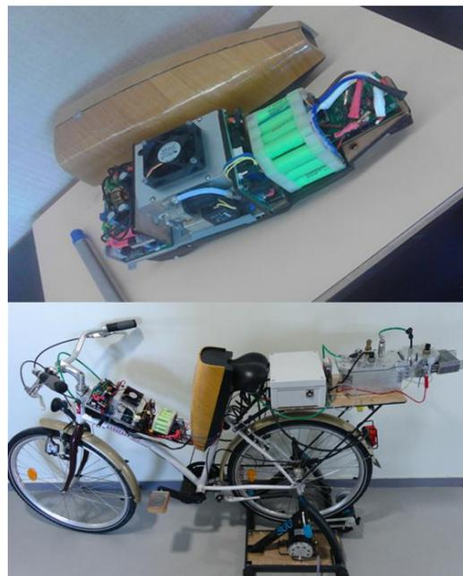
**Figure 13** Fuel cell and control kit (up) installed on the bike prototype (down).
