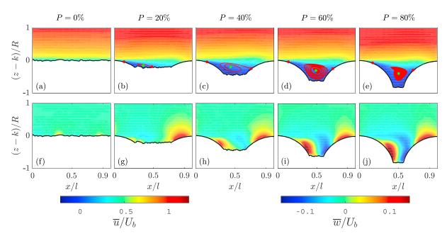
**Figure 2.** Dimensionless mean velocity fields for  $Re_D = 27,700$  (experiments PXXQ14) in plane C for all five protrusion levels P = 0-80%, with (a–e) streamwise velocity and (f–j) vertical velocity. The red dots show the position of the separation and reattachment points, and the green dots show the position of the center of the vortex. The overbar denotes time averaging.
