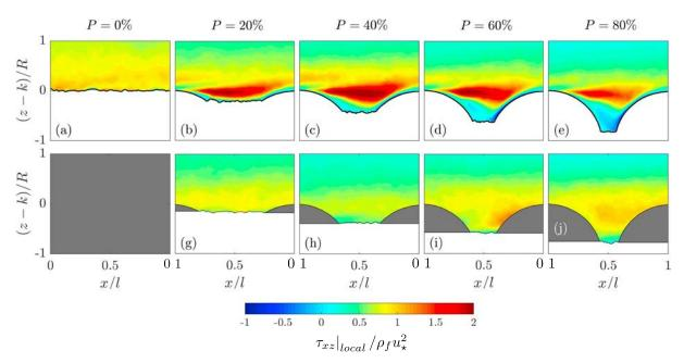
Figure 3. Dimensionless local shear stress  $\tau_{xz}|_{\text{local}}/\rho_f u_{\star}^2$  for  $Re_D=27,700$  for the different protrusion levels. (a–e) Measurements in plane C. (g–j) Measurements in plane A. Gray areas are regions hidden from particle image velocimetry measurements.
