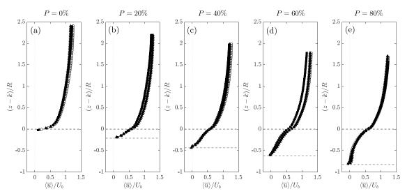
**Figure 4.** Vertical profiles of double-averaged longitudinal velocity  $\langle \bar{u} \rangle$  for  $Re_D = 27,700$  (black square),  $Re_D = 18,600$  (empty circles) and  $Re_D = 13,300$  (black triangle) and for (a) P = 0%, (b) P = 20%, (c) P = 40%, (d) P = 60%, and (e) P = 80%. The horizontal dashed lines show the height of the spherical caps and the mean altitude of the glued fine sediment.
