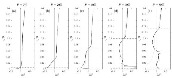
**Figure A3.** Residual shear stress between sweeps and ejections spatially averaged in the x direction in plane C (black dotted lines) and in plane A (gray lines) for  $Re_D = 27,700$ : (a) P = 0%, (b) P = 20%, (c) P = 40%, (d) P = 60%, and (e) P = 80%. Dashed lines represent the top of the spherical caps and the top of the highest fine-sediment grain.
