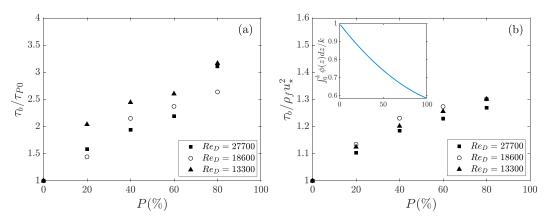
**Figure 8.** (a) Evolution of the ratio  $\tau_b/\tau_{P0}$  with the protrusion *P*. (b) Evolution of the ratio  $\tau_b/\rho_f u_{\star}^2$  with the protrusion *P*. The inset shows the evolution of the integrated porosity  $\int_0^k \phi(z) dz/k$  with the protrusion *P*.
