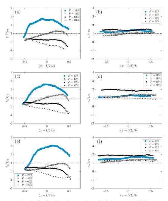
**Figure 9.** Horizontal profiles of fine-sediment shear stress  $\tau_s$  between the spherical caps, normalized with the reference shear stress  $\tau_{P0}$  (measured in the no-protrusion case P=0%) for all protrusion  $P\geq 20\%$ .  $Re_D=27,700$  in planes C (a) and A (b),  $Re_D=18,600$  in planes C (c) and A (d), and  $Re_D=13,300$  in planes C (e) and A (f). The longitudinal position is normalized by the spacing b at the base of protruding caps (Figure 1c).
