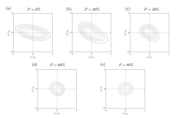
**Figure A1.** Joint probability density functions of the fluctuating velocities in a horizontal line at  $z = d_{50}$  above the fine-sediment bed in plane C and  $Re_D = 27,700$ : (a) P = 0%, (b) P = 20%, (c) P = 40%, (d) P = 60%, and (e) P = 80%.
