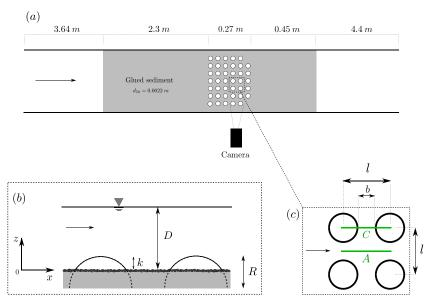
**Figure 1.** (a) Top view of the flume and positions of the patch of spherical caps (white circles) and glued sediment (gray shaded). (b) Zoomed side view of the patch. (c) Top view of an elemental pattern of spherical caps and positions of the laser sheets, *A* and *C*.
