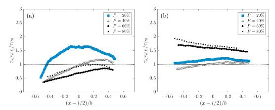
Figure 10. Horizontal profiles of fine-sediment shear stress  $\tau_{s,TKE}$  estimated with the turbulent kinetic energy between the spherical caps and normalized with the reference shear stress  $\tau_{P0}$  for all protrusion  $P \ge 20\%$  for  $Re_D = 27,700$  in (a) plane C and (b) plane C (Figure 1c).
