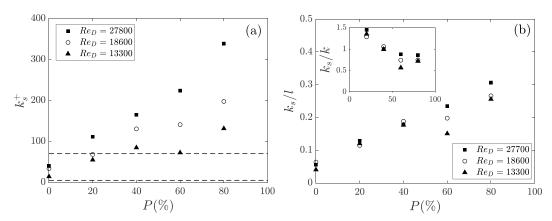
**Figure 7.** (a)  $k_s^+$  of the patch plotted against the protrusion *P*. Dashed lines delimit the hydraulically smooth, transitional and rough bed. (b) Equivalent sand roughness  $k_s$  normalized by the distance between hemispheres plotted against the protrusion *P*. The inset shows the evolution of  $k_s$  normalized by the height of the spherical caps k.
