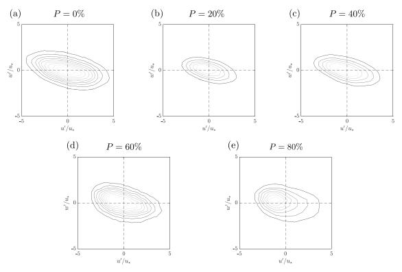
**Figure A2.** Joint probability density functions of the fluctuating velocities in a horizontal line at  $z = d_{50}$  above the fine-sediment bed in plane A for  $Re_D = 27,700$  and (a) P = 0%, (b) P = 20%, (c) P = 40%, (d) P = 60%, and (e) P = 80%.
