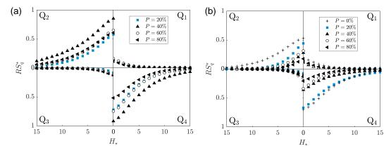
**Figure A4.** Contribution of each quadrant to the total Reynolds stress plotted as a function of the hole size for a hole based on a multiple  $H_{\star}$  of the friction velocity for  $Re_D=27,700$ : (a) at the spherical cap's top z=k and (b) at  $z=d_{50}$ .
