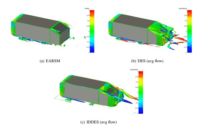
Figure 6:  $25^{\circ}$  slant angle - Vortex structures around the Ahmed body visualized by iso-surfaces of the non-dimensional Q-criterion (Q=50).
