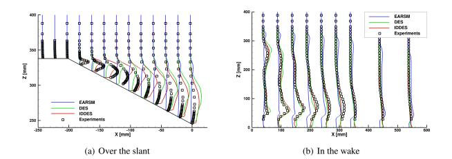
Figure 9: 25° slant angle - Turbulent kinetic energy on the rear slant and in the wake.
