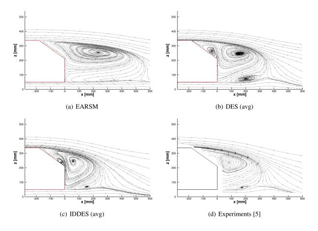
Figure 3:  $35^{\circ}$  slant angle - Streamlines in the symmetry plane Y = 0.
