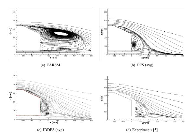
Figure 7:  $25^{\circ}$  slant angle - Streamlines in the symmetry plane Y = 0.
