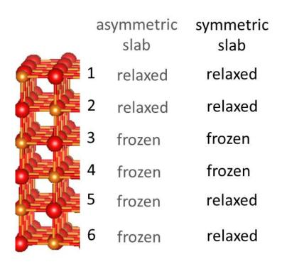
Figure 1: The slab models used in this work to study the surfaces. Layers are labelled with numbers 1-6.
