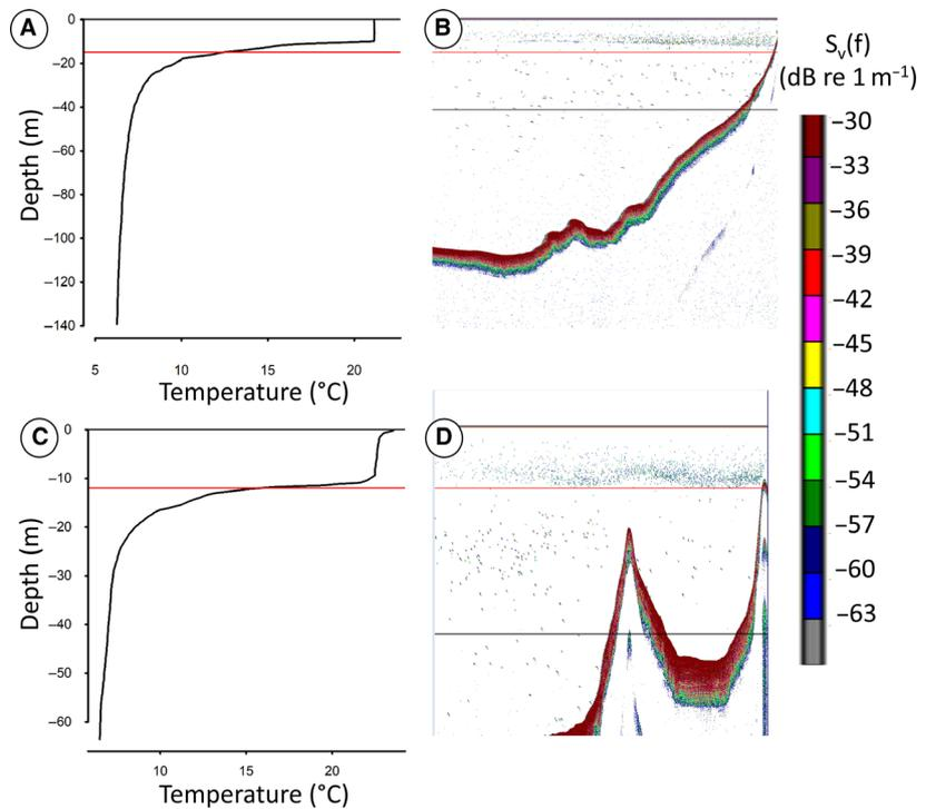
**Figure 2.** Temperature profiles (A and C) and echogram examples (B and D) in Lakes Bourget (A and B) and Annecy (C and D). The red line represents the limit between the upper and lower layers. The black line represents the lower limit of analyses.
