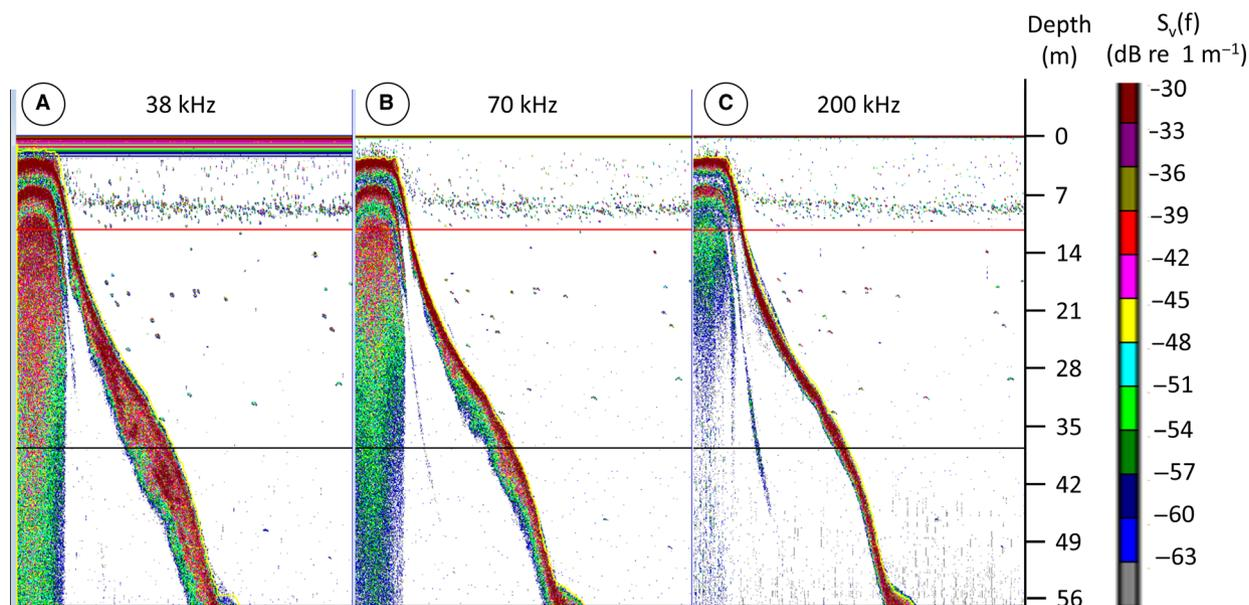
**Figure 3.** Echograms of the three frequencies (A: 38 kHz, B: 70 kHz, C: 200 kHz) in Lake Bourget. The depth scale represents the depth (in metres) and the coloured scale the mean volume backscattering strength ( $S_v(f)$  in dB). The red line represents the thermocline and the black line represents the lower limit of analyses.
